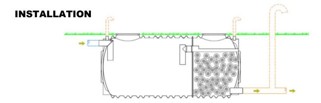
ECODEPUR® BIOFIX installation must follow the recommendations of the document supplied Installation PE Reactors/Tanks.
